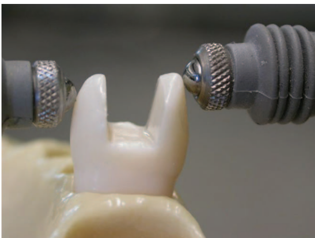
Figure 3. LVDTs connected to data acquisition system, in which the entire setup was assembled on a stabilized table to minimize noise.
